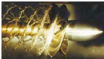
Propeller cavitation Image courtesy: http://www.rcboataholic.com/hardware/prop.htm
