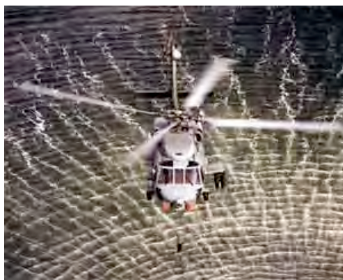
AN/AQS-22 Airborne Low-Frequency Sonar (ALFS) deployed from a US Navy MH-60R multi-mission helicopter (US Navy photo)
